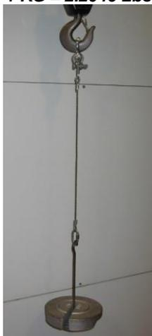
***Figure 9: Free Hanging Weight simulating cable tension.***
