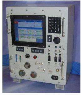
The AN/ARM-206 measures fixed or varying range and bearing performance, including search/track ability, transmitter power output, receiver sensitivity and coding and decoding parameters on all TACAN channels and air-to-air range and bearing performance.
