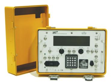
The T-36C RF output allows testing from the flight deck of most large aircraft using an expandable, omni-directional antenna. Testing of all functions can be performed with the unit-under-test (UUT) directly connected to Test Set.
