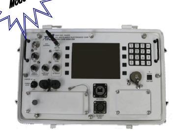
The TR-420 large 5.7 in. color LCD screen, surrounding soft-keys and keyboard provides easy and quick access to a multiple of test screens menus and display options. This enables single man operation, instant results via a host of preprogrammed and manually variable parameters to meet the most demanding requirements for testing of airborne avionic and communication equipment in both Air to Air and Direct Connect applications.
